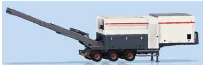
Waste shredder on a trailer basis
